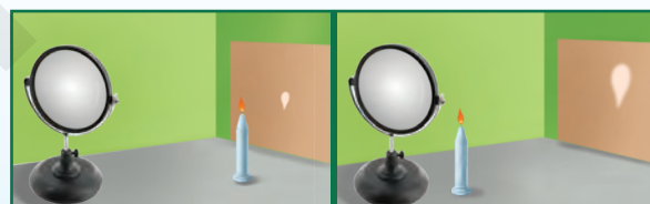
Real images formed by a concave mirror
