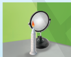
Virtual image formed by a concave mirror
