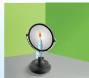
Virtual, erect and diminished image
